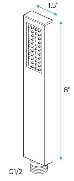
Flow Rate: 2.0 GPM / 7.6 LPM
